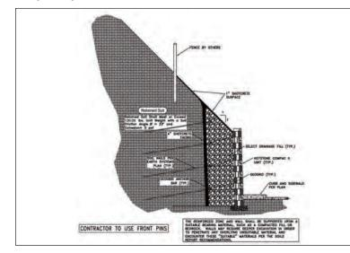
Over 16,000 square feet of Keystone Compac II units, produced by Keystone supplier RCP Block & Brick, were used on the project. The wall reached 27 feet at its highest point.
